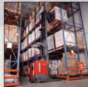
The first AC-powered *Reach-Fork®* truck built in North America was introduced in 2001, on the 50th anniversary of the first narrow aisle truck. The AC-powered truck improves productivity, increases work done per battery charge and significantly reduces maintenance costs.
