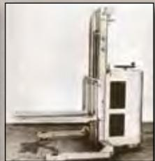
The Lyon-Raymond Model 700 SpaceMaker truck was the first electric, narrow aisle lift truck. It was able to work in aisles less than seven feet wide. Designed without a counterbalancing chassis, the vehicle preserved its gravitational integrity by straddling the pallet with baselegs, the basic principle for all narrow aisle trucks from that point on. This truck made The Lyon-Raymond Corporation the undisputed leader in the material handling industry.
