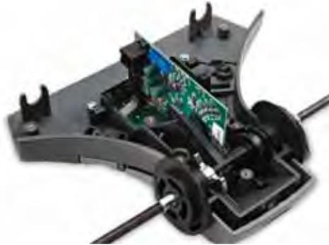
▶ Hall-effect sensors in the handle replace potentiometers, and do not contact, which minimizes wear. The CAN Bus technology eliminates 40% of wiring, minimizing time needed for wiring and troubleshooting.
